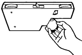
1. Disconnect refrigerator from power supply.
