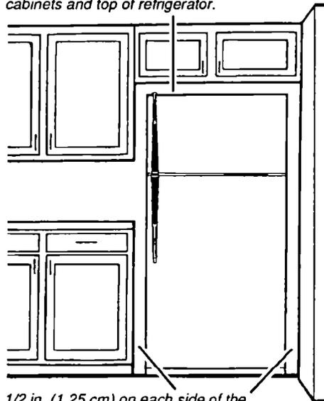
*1/2 in. (1.25 cm) on each side of the refrigerator for easier installation.*
