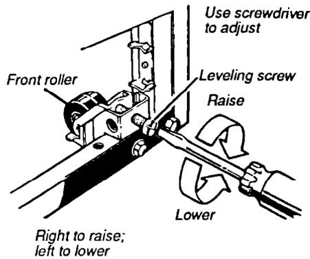
3. Check the levelness again and repeat step 2 until the refrigerator is level.
