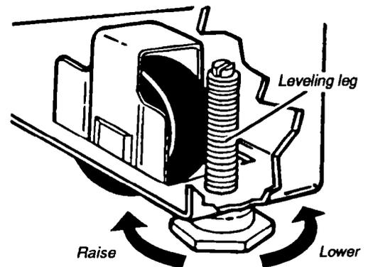
1. Two threaded leveling legs are secured into the base of the refrigerator. Remove the legs and insert them into the holes at the bottom front corners of the refrigerator. Carefully roll or slide the refrigerator into place.
