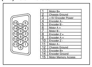
QCI recommends our QCI-C-D15P-D15S-nn (nn = length in feet) cable to interface between the motor and the controller.
