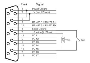
These signals provide power, communications and 3.3v IO signals (digital and analog).
