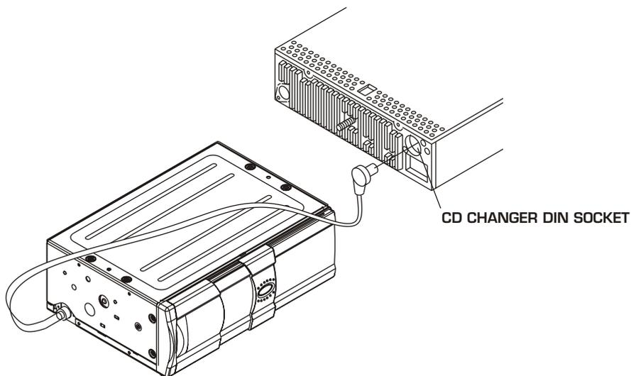
When you want to play the CD changer, plug the CD changer DIN into the socket of the back of the car audio unit.
