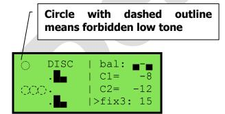
When the low tone is forbidden, upon discovering objects which provoked longer signal, a **sound is not produced**, but the signal's strength and type are displayed.
