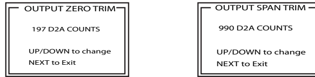
Figure 40 Configuration Menu - Output Zero Trim and Output Span Trim
