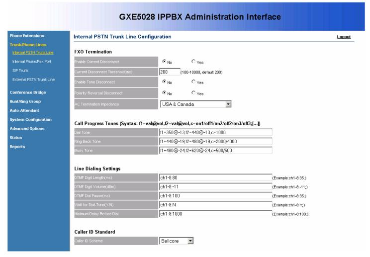
FXO Termination: Specify line disconnect signaling and impedance.
