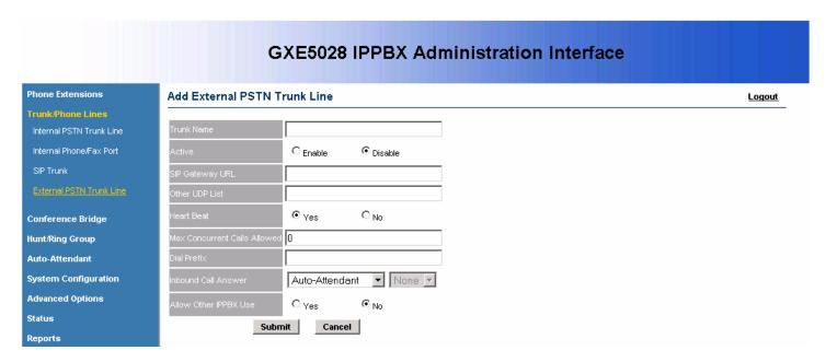
Enable the trunk: Enter a descriptive name in the Trunk Name field, and set Trunk Active to Enable.
