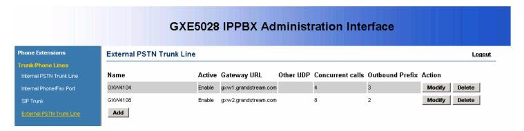
Add: Click on the **Add** button. The external PSTN trunk details page will be displayed, allowing you to enter SIP peer connection information to connect with the external PSTN trunk gateway.
