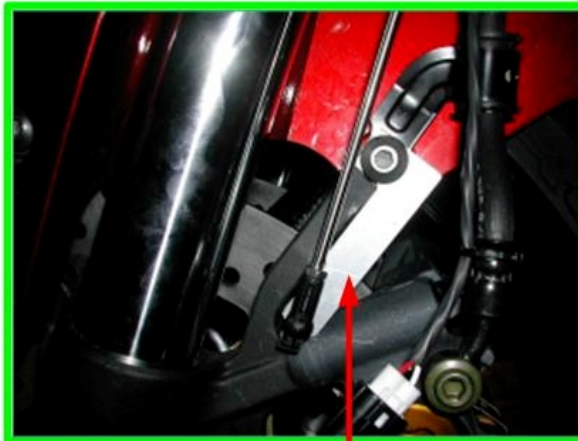
Special mounting kit to fix the lower part of the front suspension sensor
