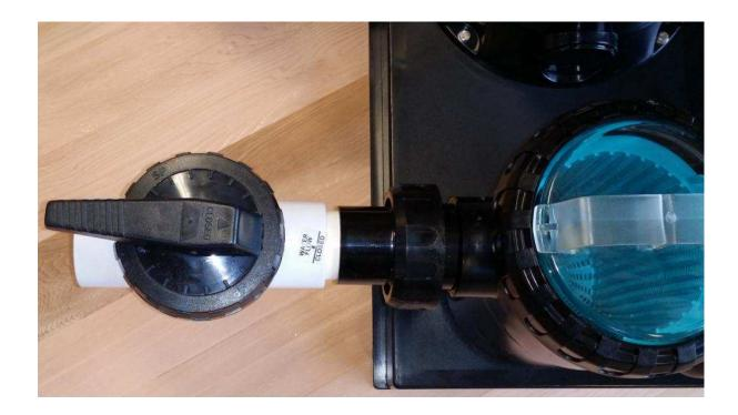
**6/** Glue the other 2-way valve into the 70mm connector PVC pipe piece with the **arrow of the water flow pointing away from the cartridge filter.** Water flows from the cartridge filter to the 2 jets.
