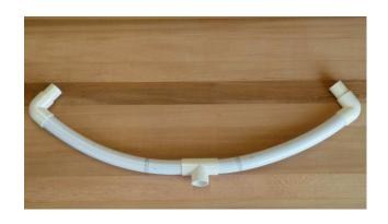
**3/** Screw tightly in the 2 Mac-union fittings onto each of the exposed pipes coming out of the pump and cartridge filter.
