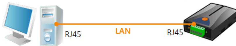
Figure 2-1 the connection between H12 and a PC
