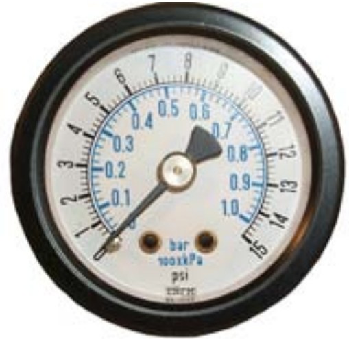
Pressure Gauge - indicates dehydrator output pressure in psig and kPa.
