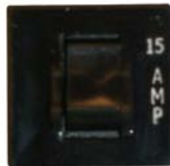
ON/OFF Switch - controls compressor and sensors. Light indicates power switch is ON.
