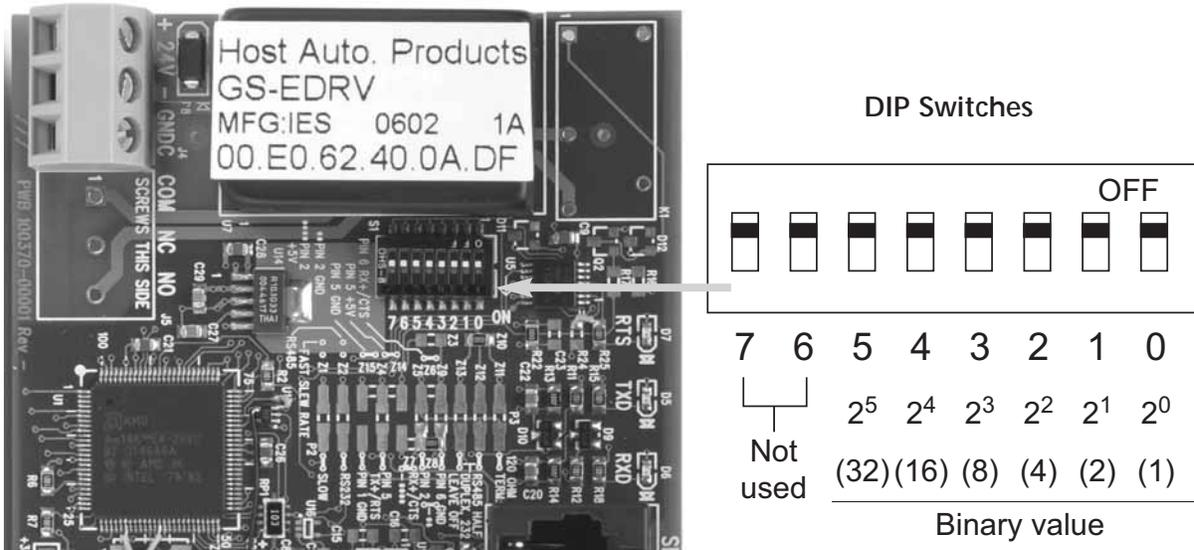
The ID equals the sum of the binary values of the slide switches set in the ON position. For example, if you set slide switches 1, 2, and 3 to the ON position, the ID will be 14. This is found by adding  $8+4+2=14$ . The maximum value you can set on the DIP switch is  $32+16+8+4+2+1=63$ . This is achieved by setting switches 0 through 5 to the ON position.
