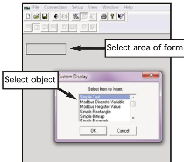
Select an object (text, charts, shapes or data) from the menu and ModScan will load the selection into the form. When creating data objects, such as Register and Discrete variables, selecting the Write Enabled checkbox (as seen on following page) will allow the user to write values out to the drive from this form.
