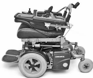
Figure 11. The attendant control can easily be removed for transport.
