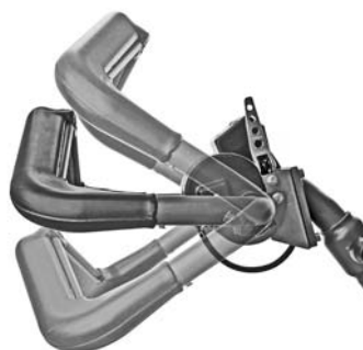
Fig. 3. Setting the steering bar angle.
