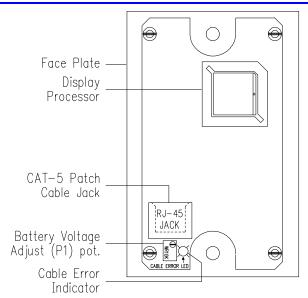
The Battery voltage calibration potentiometer is located in the lower left hand corner of the PVDM6 below the RJ-45 jack, along with a cable error LED.
