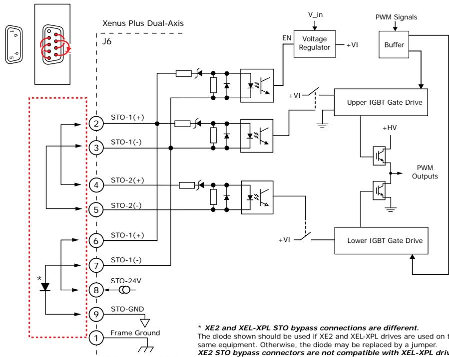
\* XE2 and XEL-XPL STO bypass connections are different. The diode shown should be used if XE2 and XEL-XPL drives are used on the same equipment. Otherwise, the diode may be replaced by a jumper. XE2 STO bypass connectors are not compatible with XEL-XPL drives.
