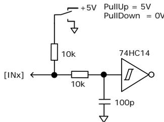
INPUTS WITH PROGRAMMABLE PULL UP/DOWN
