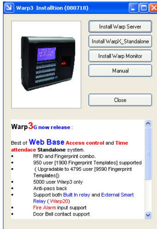
First install **WarpX\_client** program, then **Warp Server** and **Warp Monitor** after. After installed the entire program, please start WarpX\_Client program first.
