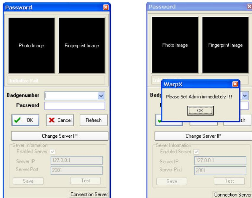
When enter the program for the first time, press [Enter] 2 times to bypass the password authentication process. The main windows will pop up.
