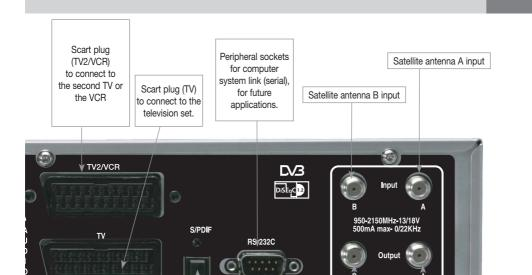
S/PDIF digital audio output. Remove the cover before use. Satellite antenna A output
