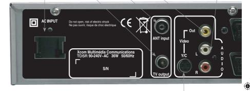
"S-VHS" outlet for an S-Video (Y/C) inlet television / Videoprojector or a S-VHS / Hi-8 video recorder.
