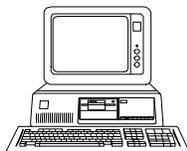
If you wish to monitor the test with a computer, connect a null modem cable to the smaller of the two "D" connectors at the rear of the instrument. Use any serial port communications program (not provided) on your computer to read the messages emitted at the MAX-1000 serial port. The content of each message can be selected from the REPORT ITEMS TO PRINT menu which is described on page 40.
