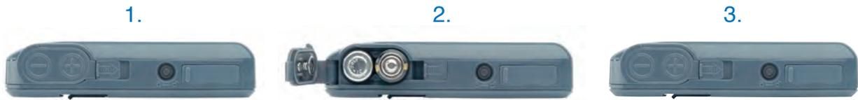
1. Remove battery cover by sliding the lock to the open position and lift the battery cover open.
