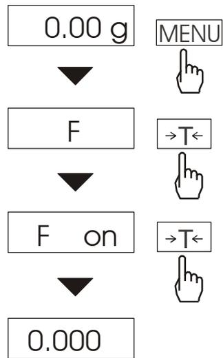
Function activation causes displaying measurement results in force units (mN).
