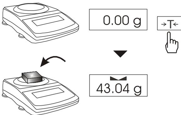
When a pan is empty and indication is different than zero press  $\rightarrow T \leftarrow$  key.
