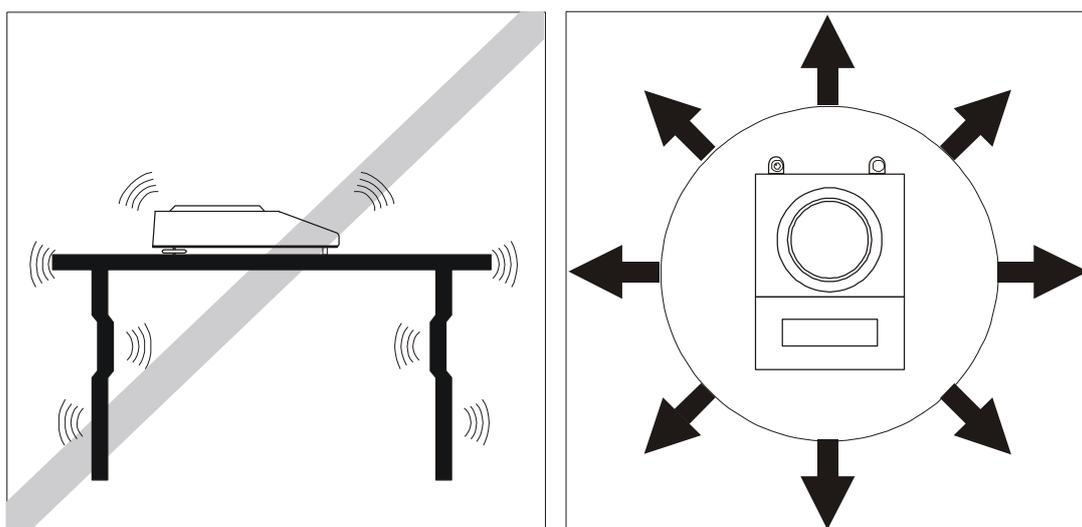
When choosing a location to set up the balance, remember the following rules to ensure proper working conditions and user-friendly operating:
