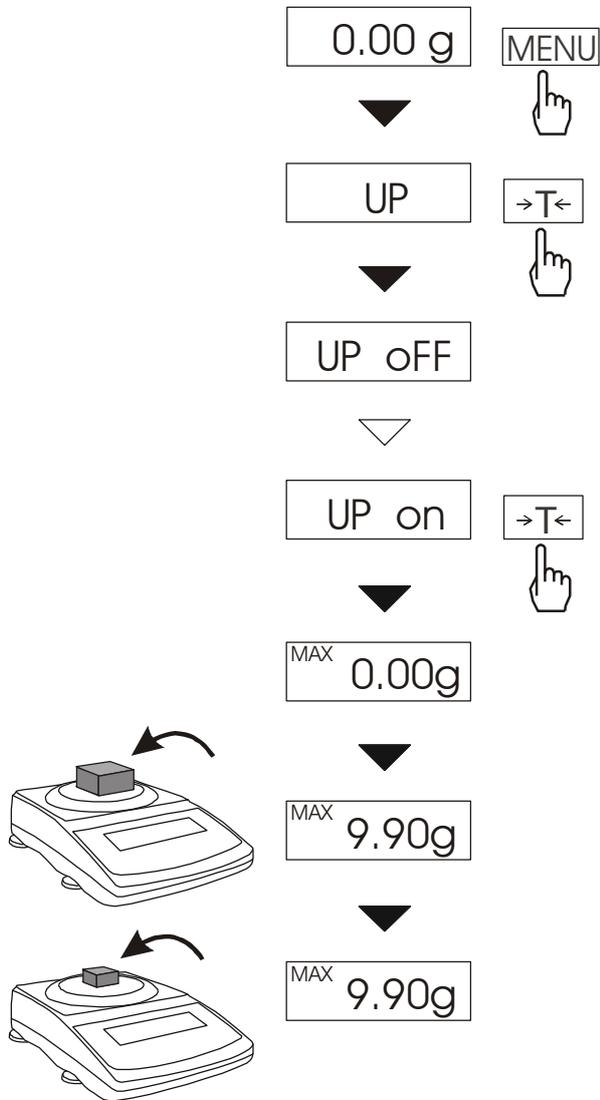
Before measurement the scale should be tared.
