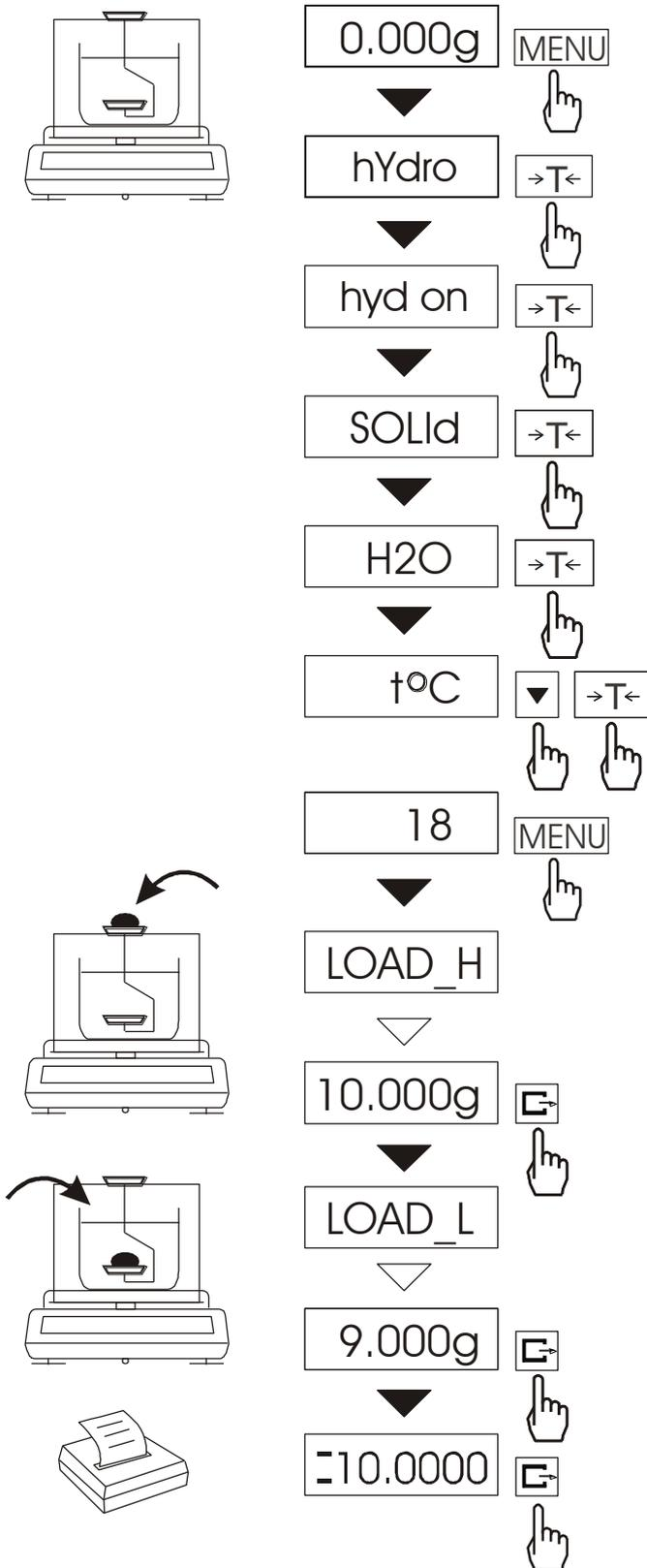
This function calculates material density basing on its weight in air and in water using the formula below:
