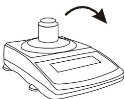
Remove a protective mark from a calibration switch at the back of a balance.
