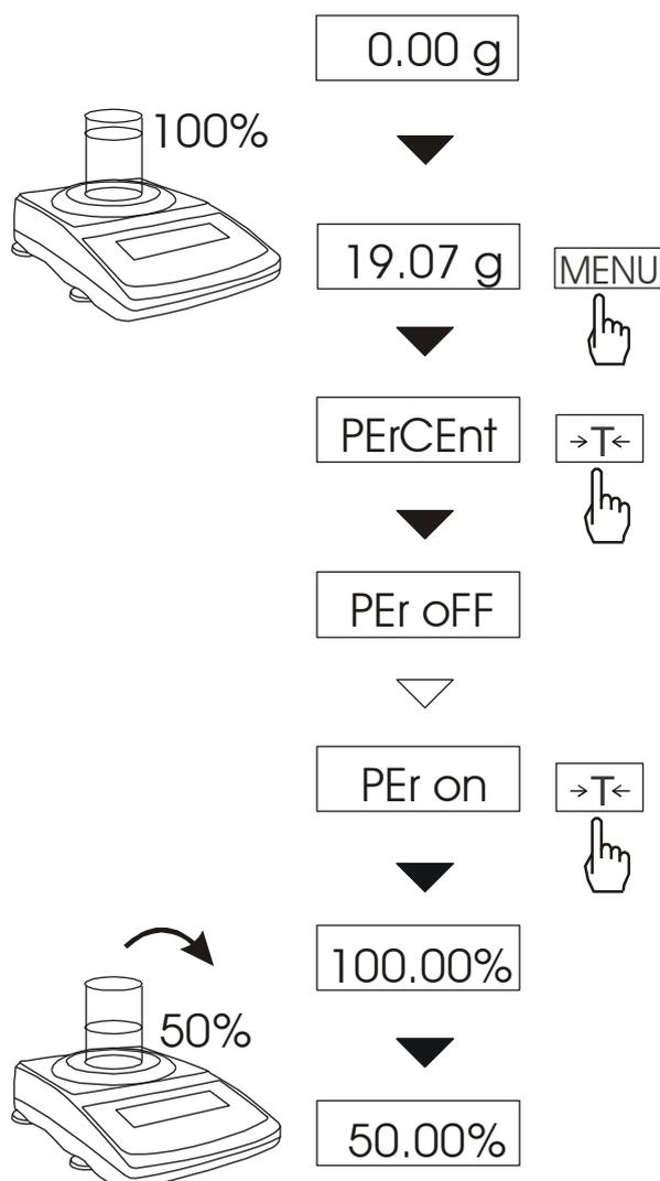
This function enables to display weighing result as a percentage of a reference sample.
