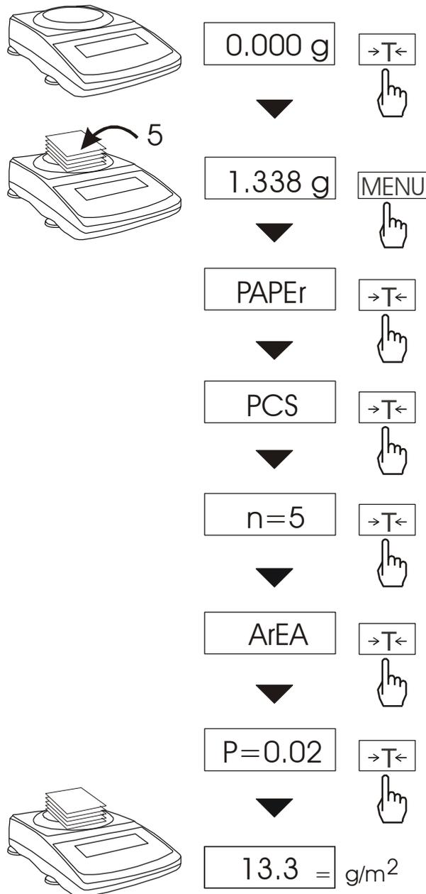
The balance must be tared just before the measurement.
