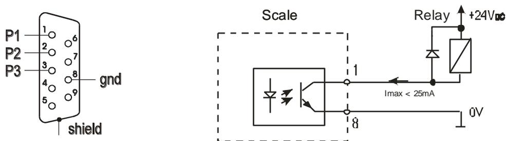
*Relays* output is the open collector transistor output with load capacity 25mA / 24V. Transmitter inputs must be protected with diodes, e.g. 1N4148.
