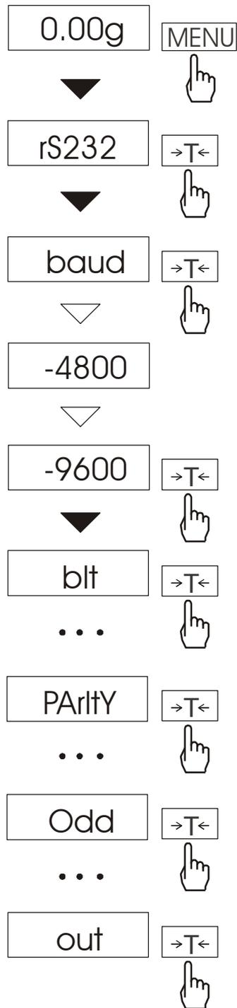
The function enables to set the following transmission parameters (standard parameters underlined:
