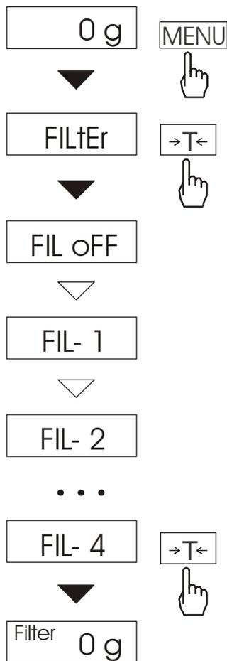
This function allows using digital filter with selected intensity during weighing. Filter reduces the influence of mechanical vibrations (air blasts, base vibrations) on measurement result.
