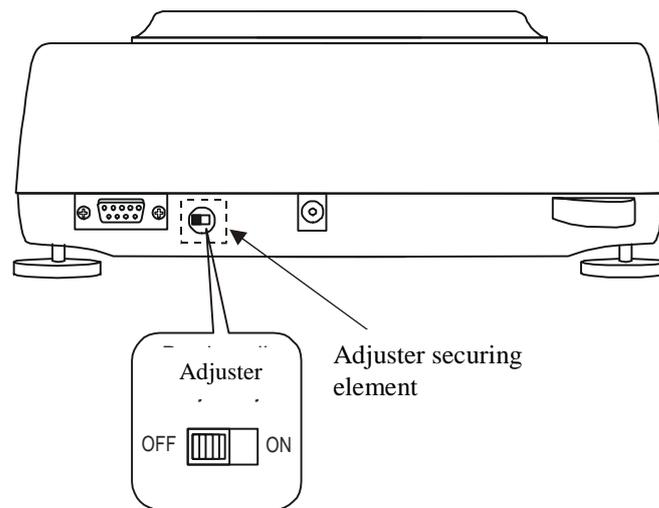
In legalized scales to perform calibration it is needed to change adjuster position. Adjuster is situated under adjuster securing element.
