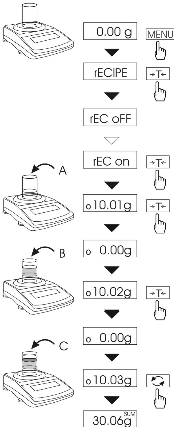
This function enable to weigh few ingredients in one container and to display aggregated sum of all ingredients.
