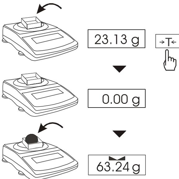
A balance is equipped with tare equal to its range.
