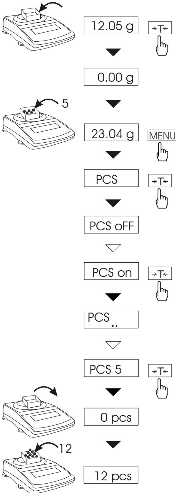
This function enables to count identical pieces, e.g. turnbuckles or buttons.
