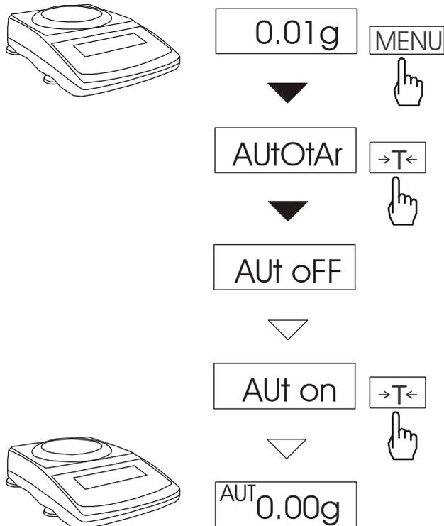
When AUtotAr function is activated, a balance automatically keeps zero indication if a pan is empty or if zero indication was acquired by pressing **→T←** key. To leave the function press **MENU** key, then with **→T←** key chose **AUtOtAr** and **AUt oFF**.
