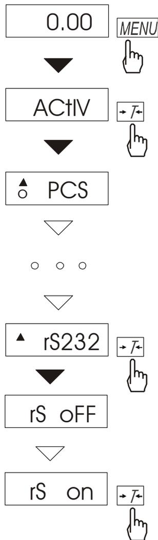
Among available user functions it is possible to select these, which should be displayed after pressing *MENU* key. It allows avoiding displaying whole list of available functions, which makes operation time longer.
