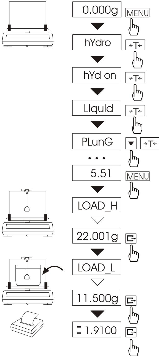
This function determines liquid density basing on plunger weight in air and in examined liquid with known volume, using the formula below:
