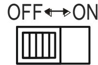
Switch to Pr ON position using small screwdriver (signalled on a display).
