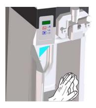
Clean both top and bottom trays, firstly, with water and then using a disinfectant solution. Wait for 10/15 minutes for it to act and rinse well with water, dry and replace it inside the fridge.
