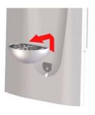
Wash the tray and the grid separately using tepid water. Dry all of the components. Replace the grid on the tray. Replace the tray in its position and press it downwards to fix it properly to the machine.
