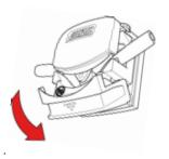
Extract the product suction tube by carefully removing it from the peristaltic pump.
