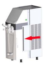
Remove the dirt and dust from the filters and replace the filters on the machine.
