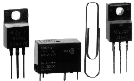
Transistor, relay and triac for PLC output circuitry. Paper clip indicates relative size.
