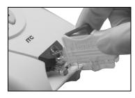
**Note**: Proper engagement of the Tenderlett Plus to the cuvette is critical to prevent a sample error.
