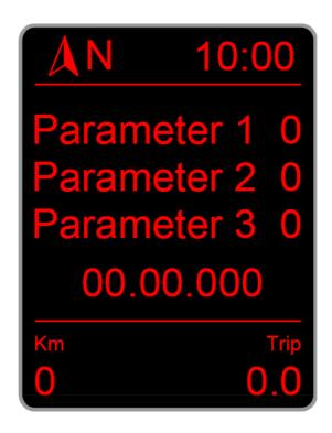
As you can see in the picture, in the top of the screen, the first 3 parameter of the active desktop are shown, and in the bottom of screen it is shown the stopwatch time. If you have any button configured for desktop change, pressing it, desktop will be changed as in the Polar FIS main screen.
