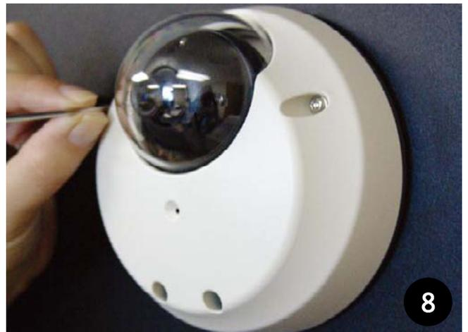
7. Adjust the camera pan and tilt. See page 11 for details. Check the LED light. Green light flickers when the camera is booting, and Red light turns on when booting is complete.
