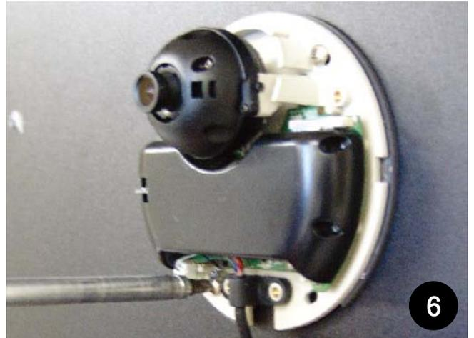
5. Pull wires through and make connections. Connect the RJ45 to a CAT5 cable or power adaptor. Refer to **"NETWORK CONNECTIONS"** for further explanation.
