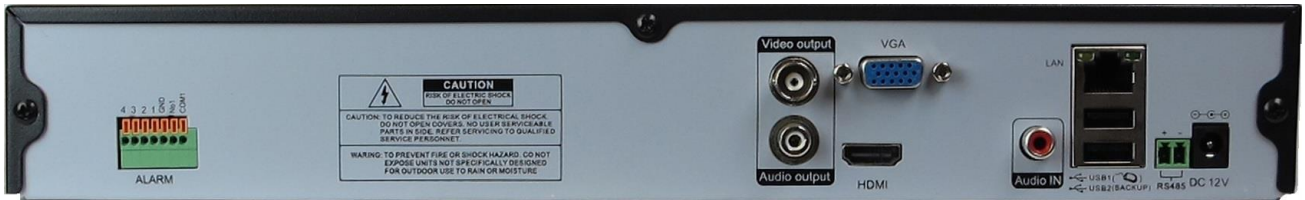
Figure 2: NVR Rear panel
