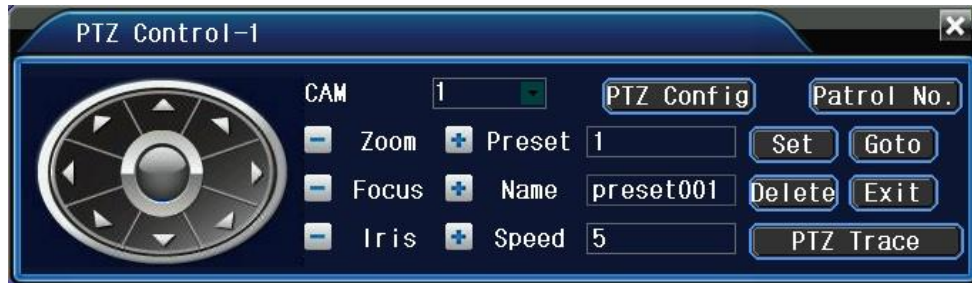
Figure 11: PTZ control Interface
