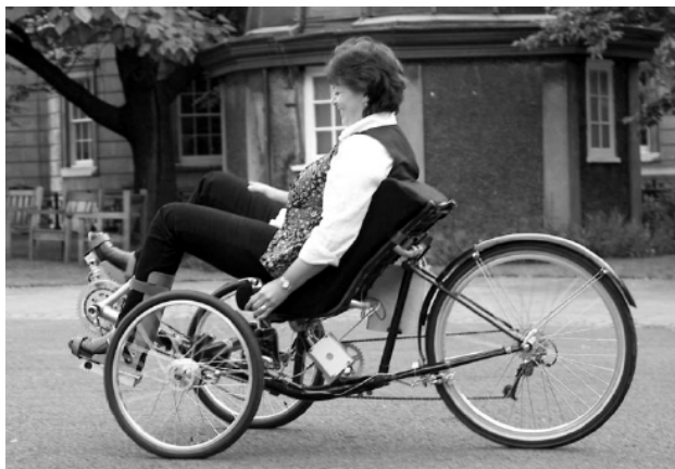
Fig 1. Paraplegic patient cycling a recumbent tricycle using an FES implant.
