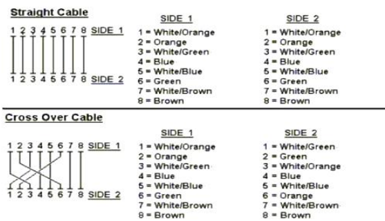
Figure A-1: Straight-Through and Crossover Cable
