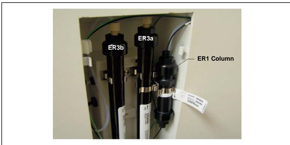
Figure 12. Mounting the ER1 Column in the RFIC-ER Compartment
