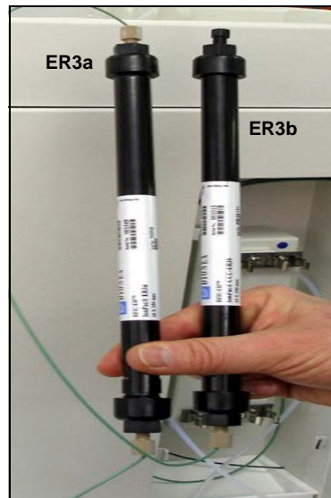
Figure 5. ER3a/ER3b Column Assembly
