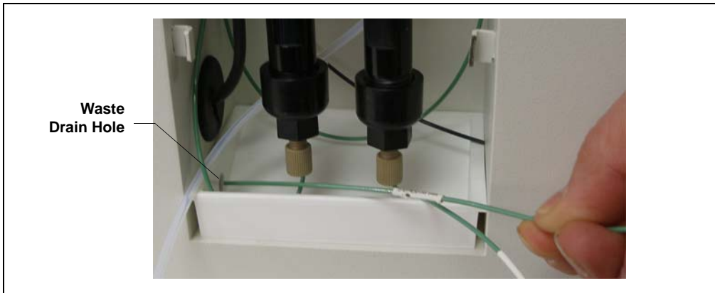
Figure 7. Routing the ER3a Column Inlet Tubing
