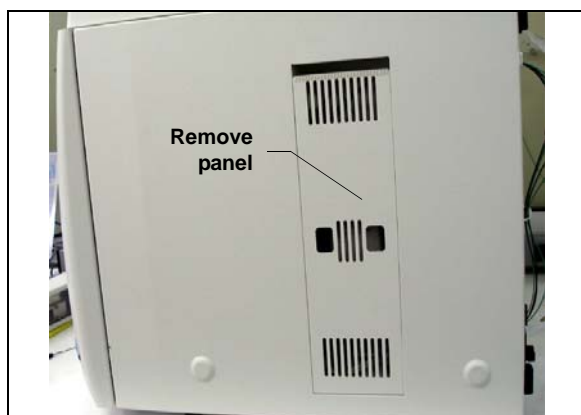
Figure 3. RFIC-ER Compartment Panel
