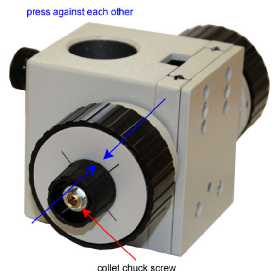
Picture 2.2: Adjustment of the stiff motion of the drive with coaxial gross and fine drive (fine drive)
