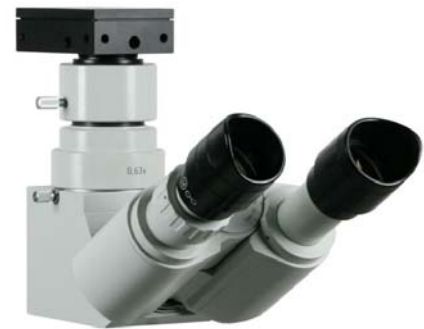
Picture 26: MZM 1 with TV-Adapter 0,63x and USB camera
