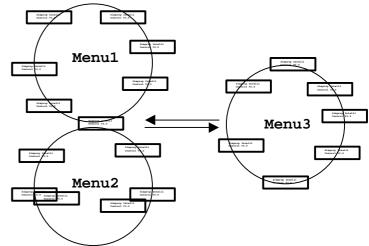
**Menu 1** On the first menu level, the charging, discharging or charge/discharge cycles are started using the [SET STOP] key. The keys [UP] or [DOWN] are used are used to select the particular charge or discharge programme.
