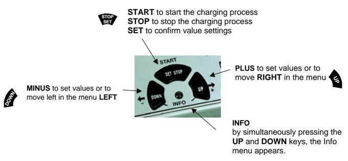
Operating the Intelli-Control V3 is extremely simple. The arrangement of the keys corresponds to the positions of the following menus and functions. The Intelli-Control V3 is divided into three menu levels. In these levels you can select the function using the [UP] and [DOWN] keys. The menus are always built in a circular form so that by pressing one or other of the keys a number of times, you come back to the starting point. The key [SET STOP] starts, stops or confirms actions.
