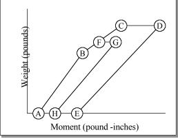
If the aircraft manual plots the weight and balance curves with weight on the vertical axis and **moment** on the horizontal axis, convert the data to the other format. In order to convert the moment to arm, simply divide by the corresponding weight.
