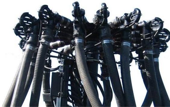
Figure 5: 1.25-inch flow sensors installed on a manifold
