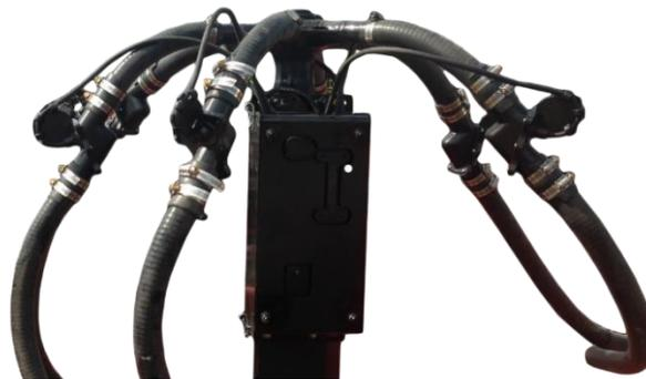
Figure 7: 1.5-inch flow sensors installed on a manifold
