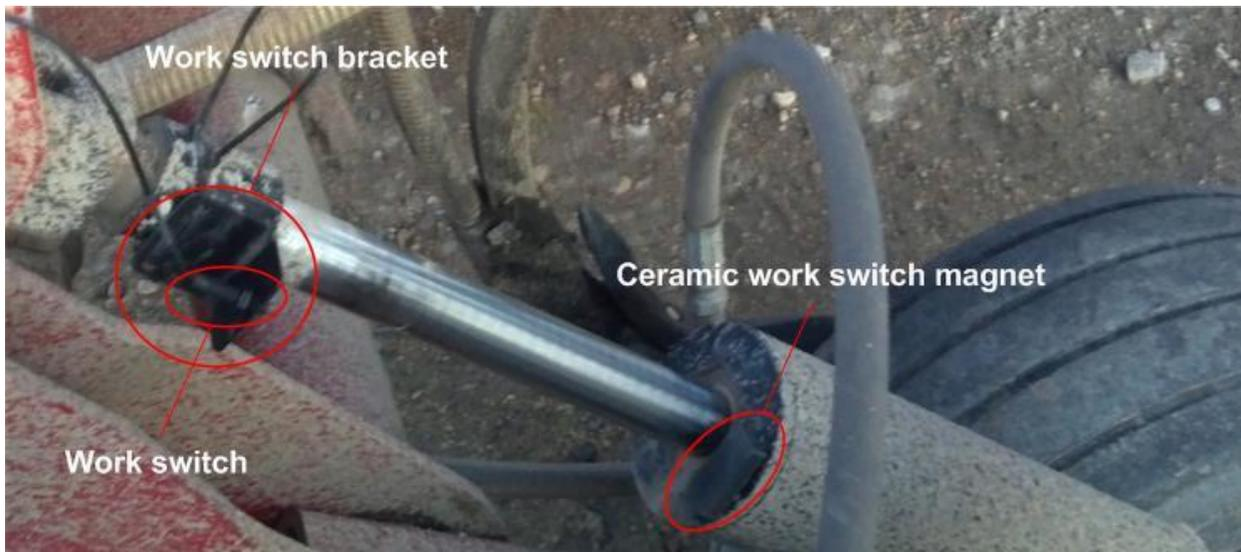
**Figure 15: A work switch installed on an implement where no bracket previously existed**
