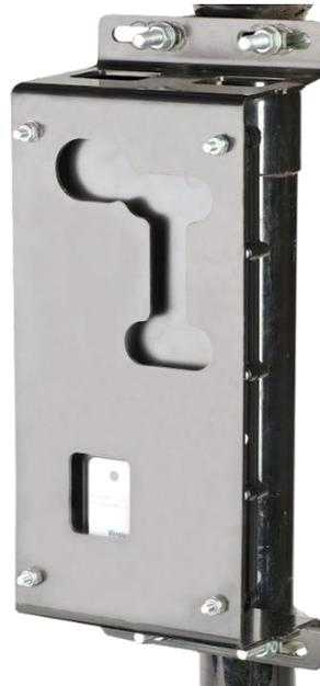
Figure 4: ECU installed on an implement tower
