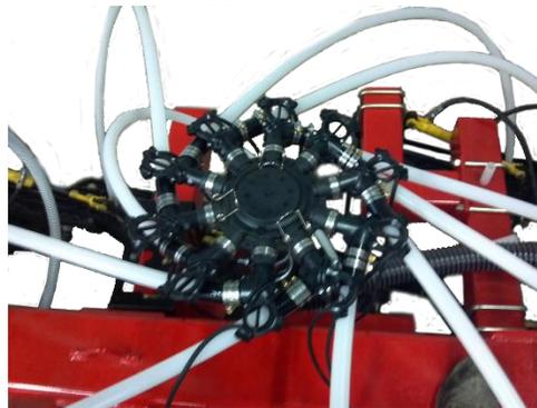
Figure 6: 1.25-inch flow sensors installed on a manifold (alternate installation)
