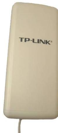
Figure 16: Wireless Blockage and Flow Monitor Access Point
