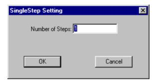
When the command is activated, a dialog box will appear on screen prompting the number of steps (program lines). Enter the number of steps and press **Enter** key or click **OK** button to set the value.
