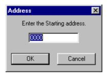
Key in the starting address and then click **OK** button or press **Enter** key to start loading. The status of program loading is displayed in a separate message box.
