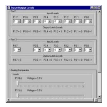
All I/O pins have three options: Level **0**, Level **1**, and **NO CONNECTION**. You can leave any I/O pin open as you do in real time. Depending upon your output selection, all output conditions are promptly indicated in the window. If you leave any I/O pin in NC, then corresponding input represents the output latch level.
