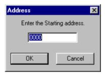
Press **OK** button after entering the starting address. The status of this binary file loading is indicated by another window.
