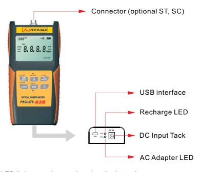
Recharge LED lights up when recharging the batteries. AC Adapter LED lights up when recharging finishes
