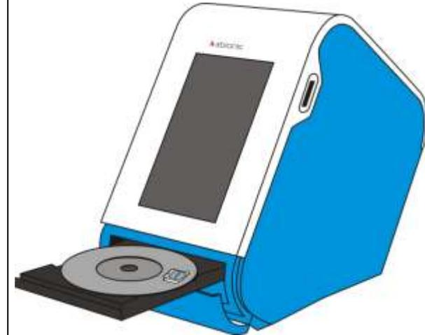
When placing the abioDISC in the disc tray, make sure that the capsule is correctly set in the abioDISC, and that the abioDISC is the correct way up as per the above diagram). Never use a defective capsule (e.g. one that is leaking or cracked etc.). Please follow steps 1 to 3 of the analysis procedure in order to open abioSCOPE disc tray.
