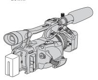
2 With the ▶ mark on the DC plug facing the cassette compartment, connect the AC Adaptor to the DC IN jack on your camcorder.
