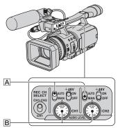
1 Set the AUTO/MAN switch A of the channel to be adjusted to MAN.
