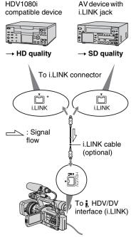
\* An i.LINK jack which is compatible with HDV1080i specification is required.
