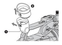
2 Remove dust from inside the viewfinder and the part shown below with a blower.
