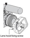
Align the marks on the lens hood to those on the camcorder, and turn the lens hood in the direction of the arrow. Tighten the lens hood fixing screw.
