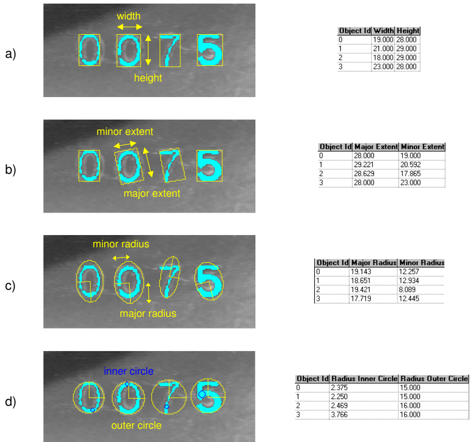
Figure 1.3: The extent of a blob: (a) along the image axes; (b) the extent of its smallest surrounding rectangle; (c) the radii of its equivalent ellipse; (d) its inner and outer circle.
