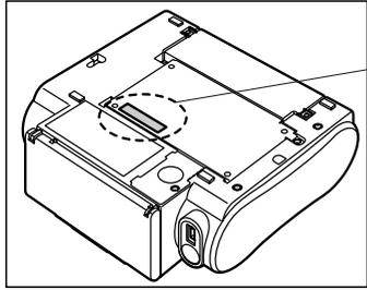
The serial number is located on the backside of the printer.
