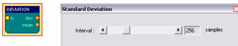
This Element calculates standard deviation and mean of  $n$  samples and puts the results to the output ports. The number of samples for the calculation interval can be set using the slider bar.
