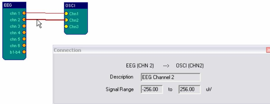
By left-clicking a connection, a dialog with information about the connection is displayed. It states the connected ports, a description of the signal and the signal-range.
