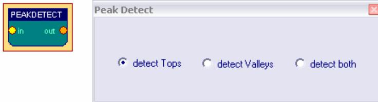
The *Peakdetect* - element detects extreme-values (signal tops or signal valleys) and outputs these values.
