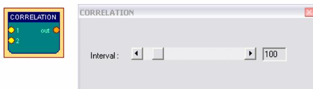
This element calculates the cross-correlation between the two signals connected to input 1 and input 2 in a selectable *Interval* of samples. Correlation is a measurement for the linear relationship between the two signals. The output will be between 1 (fully correlated) 0 (uncorrelated) and -1 (fully inverse correlated).
