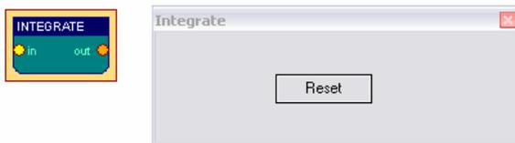
The *Integrator* element continuously sums the incoming values. Pressing *Reset* sets the buffer to zero, this is also done when starting or resetting the session.
