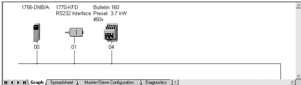
2. Right-click the DeviceNet scanner (MAC ID 00 in [Figure 6.9](#)) and select **Properties**. The Scanner Module dialog box appears.
