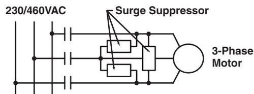
For 3-phase apparatus, a suppressor is needed across each phase
