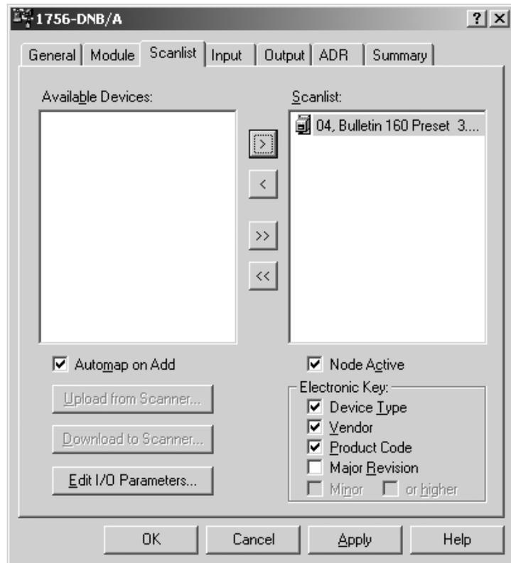
7. In the “Scanlist,” select the drive, and then click **Edit I/O Parameters**. The Edit I/O Parameters dialog box ([Figure 6.11](#)) appears.
