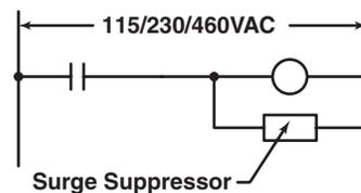
For large apparatus (electro-mechanical brakes, contacts up to size 5)
