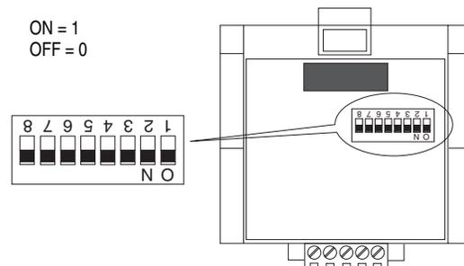
**Important:** When setting the Communication Module's *addressing* DIP Switches, make sure that each serial device on the network has a unique address. Also, all devices connected to the network must be set at the same baud rate.
