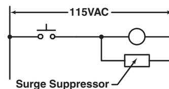
For small apparatus (relays, solenoids, and motor starters up to size 1)
