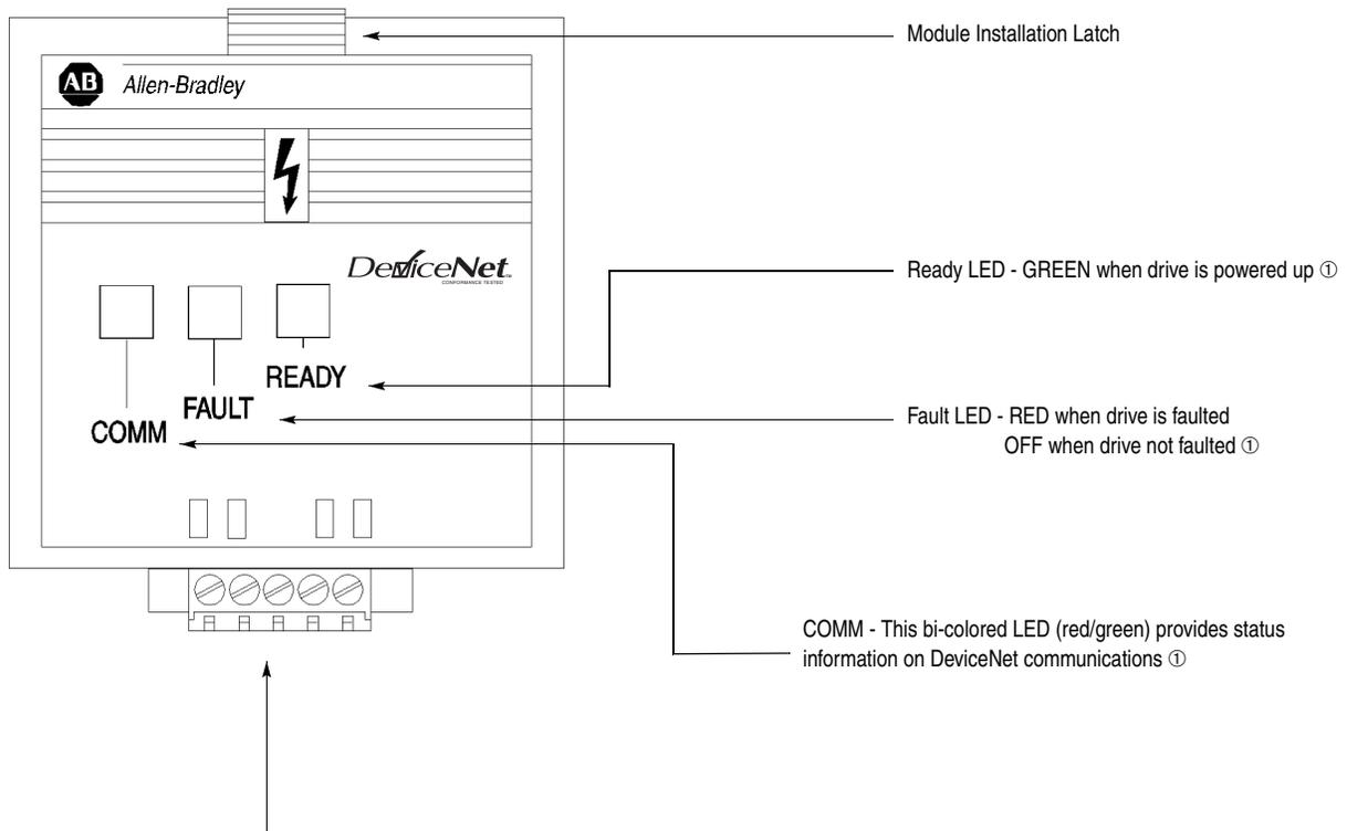
DeviceNet Terminal Block Plug - The Communication Module receives power and communications through this connector.
