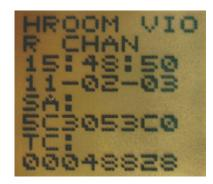
Pressing the **UP** and **DOWN** keys scrolls through the individual errors. Errors are sorted by time and date in ascending order.
