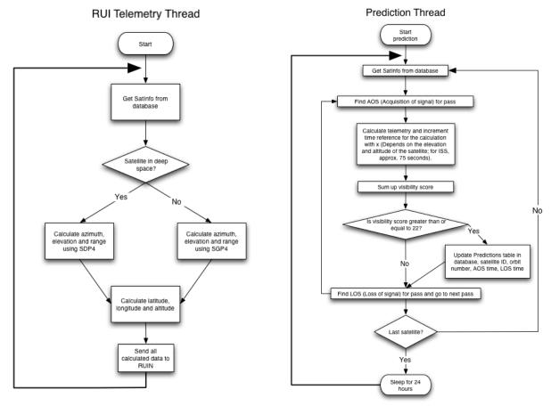
Figure 8. Telemetry and Prediction Threads.
