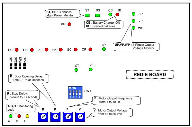
Input : ST-RS: 3-phases main power; ZF: Stop switch input (Z1-Z2); 4P: 4<sup>th</sup> pole input; CT: Contactors control input .
