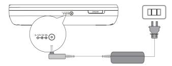
→ The charge indicator turns on. It takes less than 6 hours to fully charge the battery.
