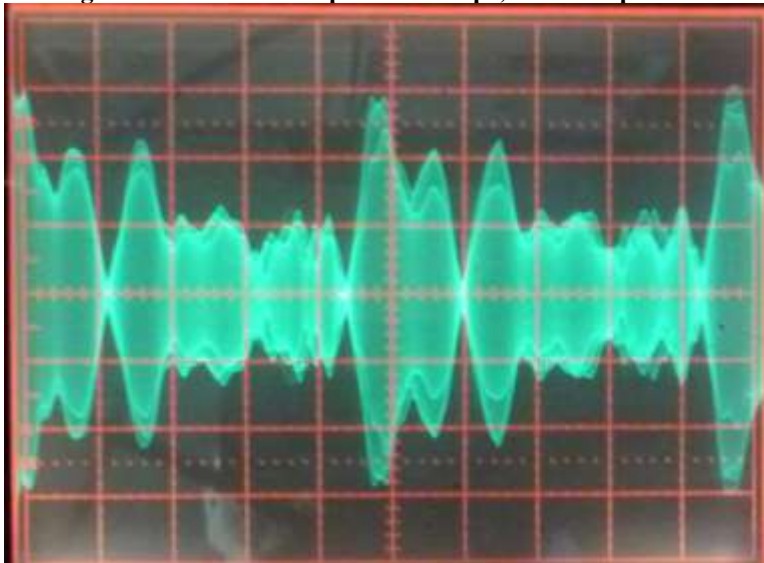
Figure 17: 100W PEP speech envelope, 6 dB compression.
