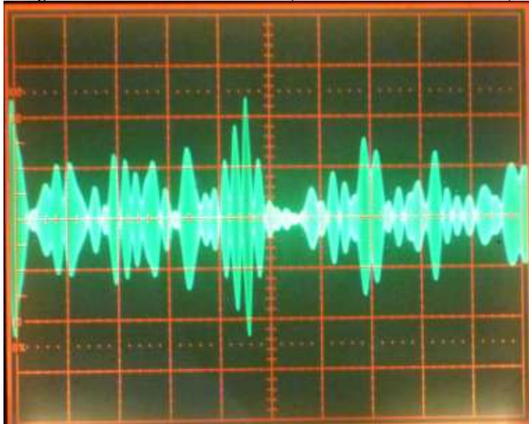
Figure 18a: 50W white noise test ( \pm 2.25 vert. div. = 50W PEP).
