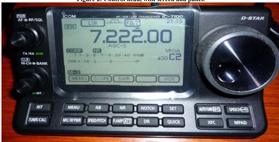
Figure 2: Control head, with screen and panel.
