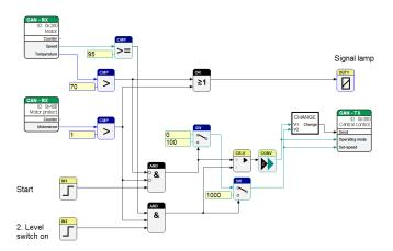
Programming the STG-650 follows using the USB port of your PC with installed miCon-L software suite and the VK-16 USB Connection Cable. The miCon-L Software supports full simulation and visualisation operation modes. miCon-L provides a variety of visualisation blocks and interactive elements to control and debug the Mini-PLC.
