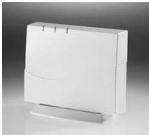
The ORiNOCO Access Point 500 connects the wired and wireless networks.
