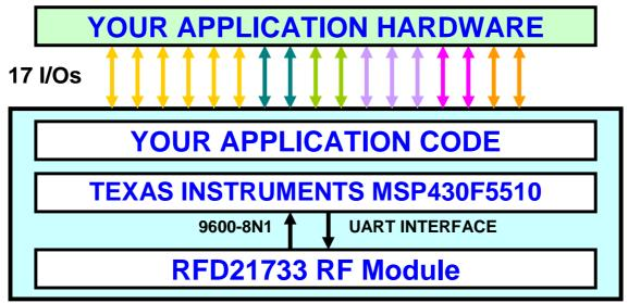
The RFD21733, with its built-in Patent Pending RFDP8 protocol provides a virtual wireless 9600-8N1 UART serial-interface to you. Any bytes you output from one module is accurately received by the receiving module(s).
