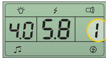
*The number in the right box indicates which monolight is being adjusted*
