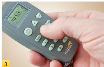
Release the TEST button on the flash head. Press 1 on the remote and then immediately press the MODEL button. A beep will sound to confirm synchronization of the remote with monolight #1.
