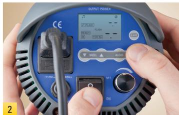
While pressing the TEST button on the flash head, switch the flash head back ON. The display will light but will display “---” instead of digits.
