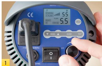
Switch the flash head on and turn the flash power regulator until you get 5.5 on the LCD screen. Turn the flash head OFF.
