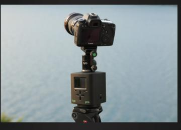
Using a Syrp Link cable matched to your camera model, connect the 2.5mm end to the camera port on the Gene, and the other end to the remote input on your camera.
