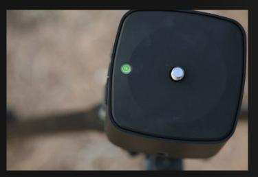
To attach your camera to the top of the Genie you can either use a tripod head, or a ball head. Screw this down securely tothe top of the Genie.
