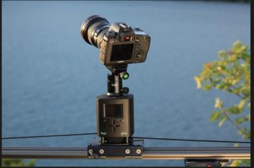
Using a Syrp Link cable matched to your camera model, connect the 2.5mm end to the camera port on the Gene, and the other end to the remote input on your camera.
