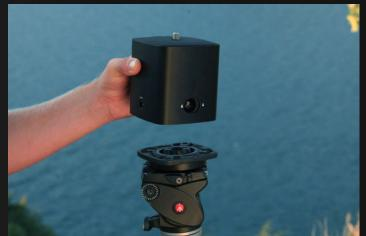
Once the Genie is in place you should check that the bubble level on the top of the Genie is showing the air bubble is in the centre of the ring. This will ensure that your shots will rotate perfectly flat.
