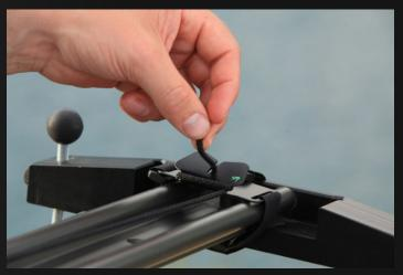
Click the Genie into the linear accessory firmly and check that the relaese catch is completly closed.
